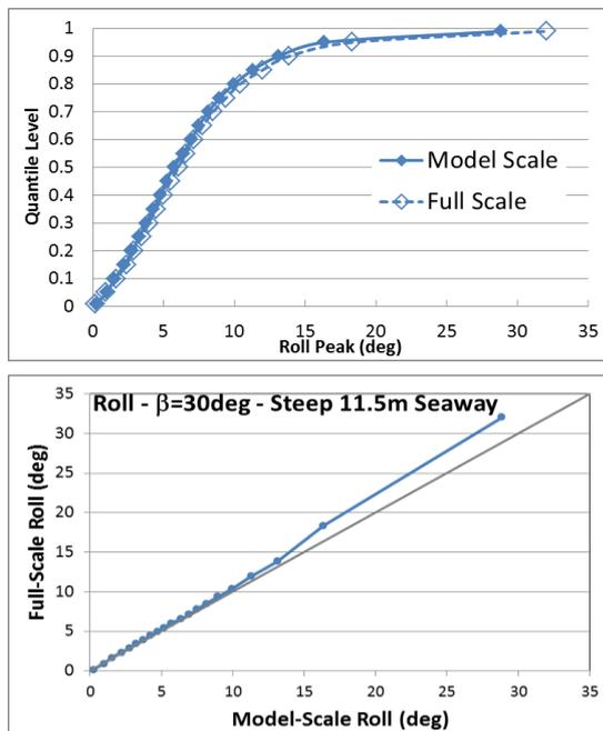
Fig. 8: Roll quantile comparisons for  $H_s = 11.5\text{m}$ ,  $T_m = 12\text{s}$  at 5 kt,  $30^\circ$  relative wave heading, between model scale and full scale. Quantile plot shown at top and Q-Q plot at bottom.
