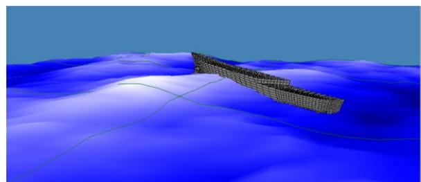
**Fig. 4:** Screen capture of simulation showing short-crested irregular sea environment.
