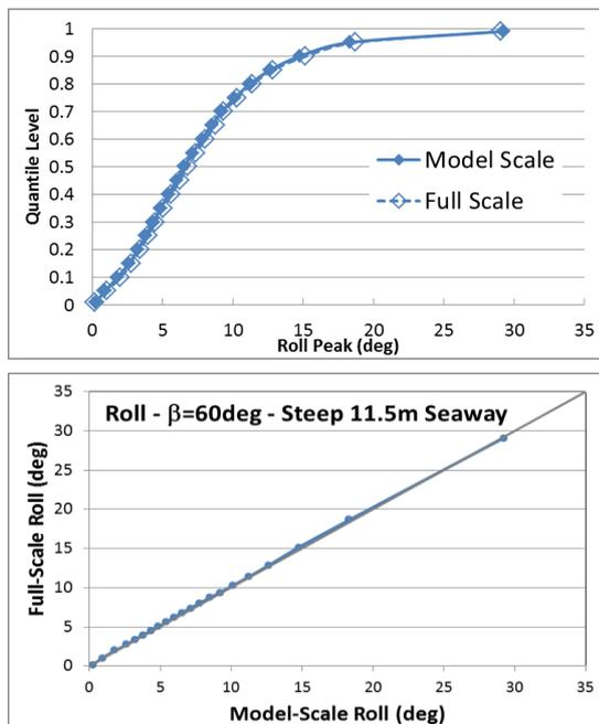
Fig. 9: Roll quantile comparisons for  $H_s = 11.5\text{m}$ ,  $T_m = 12\text{s}$  at 5 kt,  $60^\circ$  relative wave heading, between model scale and full scale. Quantile plot shown at top and Q-Q plot at bottom.
