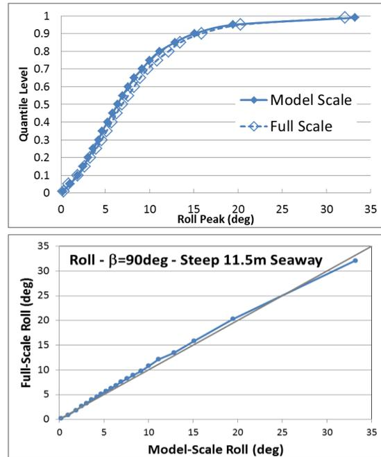
Fig. 10: Roll quantile comparisons for  $H_s = 11.5\text{m}$ ,  $T_m = 12\text{s}$  at 5 kt,  $90^\circ$  relative wave heading, between model scale and full scale. Quantile plot shown at top and Q-Q plot at bottom.
